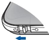
When the device is in sleep mode, Wi-Fi will be disabled and the mobile data connection will be disconnected. To have the device enter sleep mode, make sure the OLED display is on, slide the power switch to the WPS icon (↻) and release. To get the device back to normal mode, turn on the OLED display, slide the power switch to the WPS icon (↻) and release.
