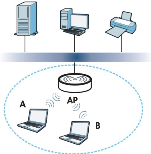
The wireless network is the part in the blue circle. In this wireless network, devices **A** and **B** use the access point (**AP**) to interact with the other devices (such as the printer) or with the Internet. Your WAH7706 is the AP.
