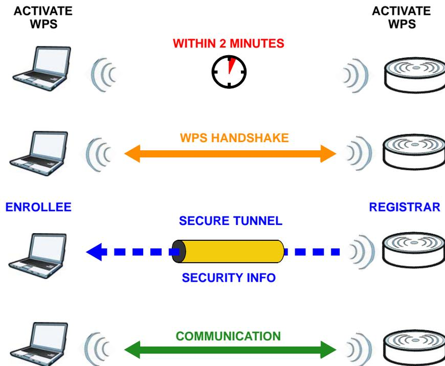
The roles of registrar and enrollee last only as long as the WPS setup process is active (two minutes). The next time you use WPS, a different device can be the registrar if necessary.
