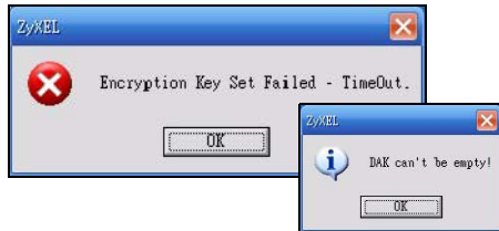
Figure 30 Incorrect DAK or No DAK
