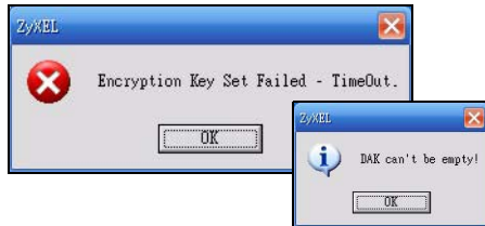
Figure 30 Incorrect DAK or No DAK
